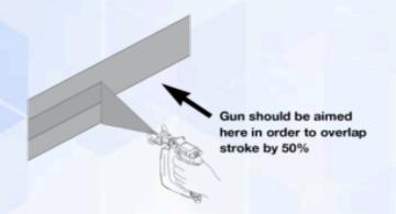
• The applicator should spray with an "X" out technique, 2 light passes at once (wet on wet) with one pass side to side and the next pass up and down. This technique helps to ensure a uniform coverage over the sometimes uneven surface of the SPF. Passes should not be confused with coats which require 4 hour dry time in between as opposed to a wet on wet pass.
