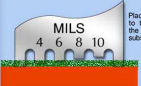
Place the gauge at ninety degrees to the coated substrate and be sure the gauge is firmly in contact with the substrate.
